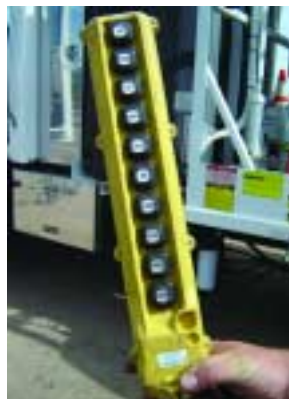
ABOVE: Most vacuum trucks have some type of vacuum relief valve that you can open from the operator's remote control. Opening this valve effectively dumps vacuum pressure and is an important safety feature. LEFT: This is a typical remote used by the vacuum truck operator. The control for the mounted relief valve is on this remote.
