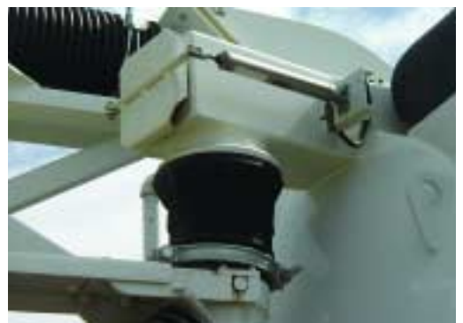
ABOVE: Most vacuum trucks have some type of vacuum relief valve that you can open from the operator's remote control. Opening this valve effectively dumps vacuum pressure and is an important safety feature. LEFT: This is a typical remote used by the vacuum truck operator. The control for the mounted relief valve is on this remote.
