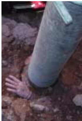
The standard tip can cause injury to a live patient. An air knife would speed up trench rescue operations and allow the tip to work in a sump created next to the patient.
