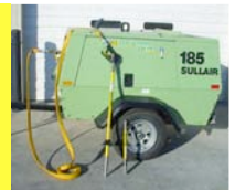
This is a typical municipal sewer cleaner and air compressor
