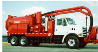
This is a typical municipal sewer cleaner and air compressor
