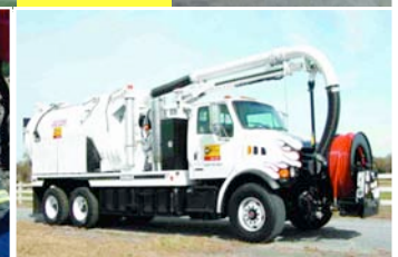
This is a typical municipal sewer cleaner and air compressor
